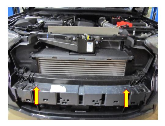
6. Using a pozi drive screwdriver to remove remove the four fasteners attaching the inner arch of the bumper to the splash guard.. This is the same for both sides.
