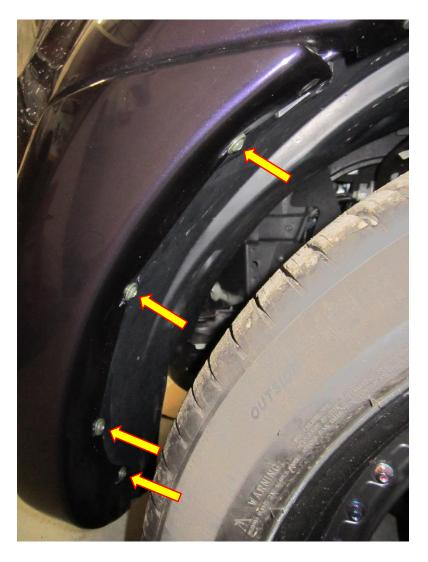
7. Locate and remove the four fasteners at underside of the bumper.
