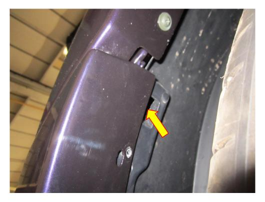
9. With the bumper now free from the vehicle there are three plugs which need unfastening. Simply press in the tab and pull to release them.
