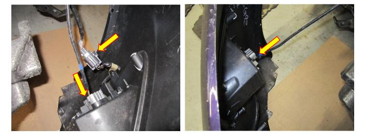
**10**. Using a 10mm socket and ratchet remove the four M6 fasteners attaching the plastic shrouds each side of the intercooler.
