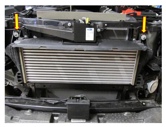
**13**. Un-clip both boost hoses going to the intercooler, with the use of a flat blade screwdriver slide the retaining clip down then pull the boost pipe from the intercooler.
