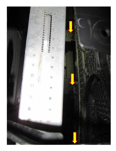
3. Using a 10mm socket and ratchet remove the two M6 fasteners attaching the top of the grill to headlights.
