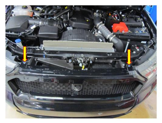
4. Locate and use a Pozi drive screwdriver to remove the two fasteners attaching the bottom of the grill. The grill will now come away from the bumper.
