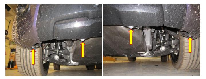
8. Remove the fastener from the inside of the splash guard attaching the bumper to the wing, do this on both sides. The bumper should now pull away from the vehicle.
