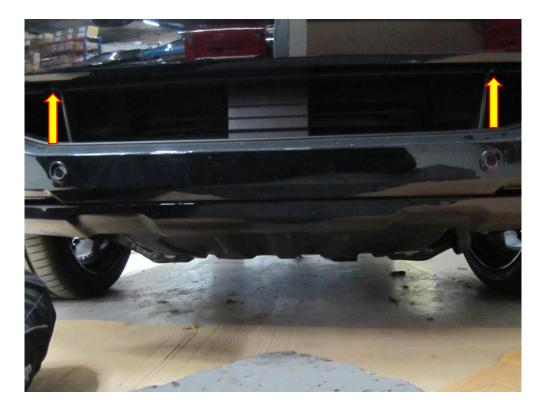
5. Remove the two plastic fasteners in the picture below with the aid of a trim removal tool or a flat blade screwdriver.
