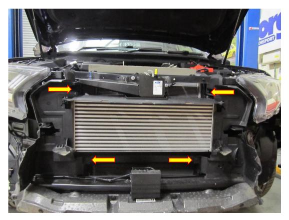
Use a flat blade screwdriver or trim removal tool to remove the plastic fasteners in the middle of each shroud
