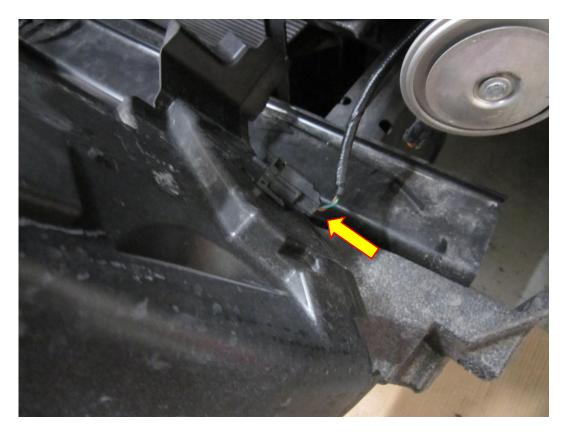
12. Remove the M6 nut and washer securing the intercooler to the vehicle. Use a 10mm socket and rachet to do this.
