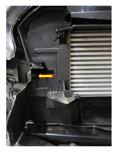
**11**. Un-plug the temperature sensor attached to the plastic shroud.
