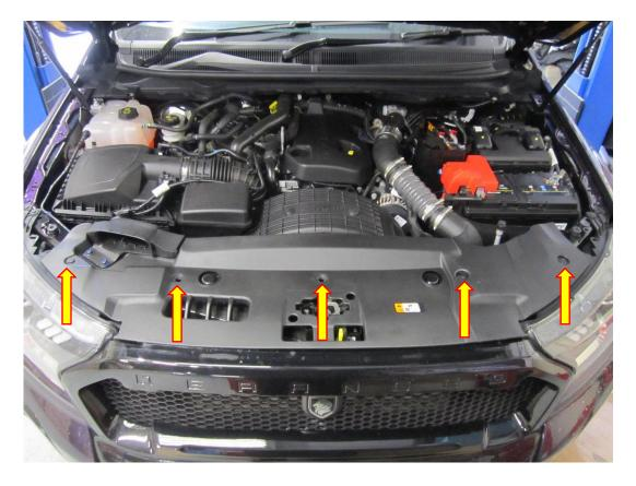
2. Use a T30 Torx drive to remove the two fasteners which attach the air scoop to the slam panel. You will now be able to remove the slam panel cover complexly.
